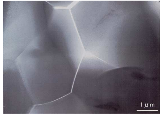
Fig. 3. Transmission electron micrograph of the as-irradiated Al 15 N specimen.
