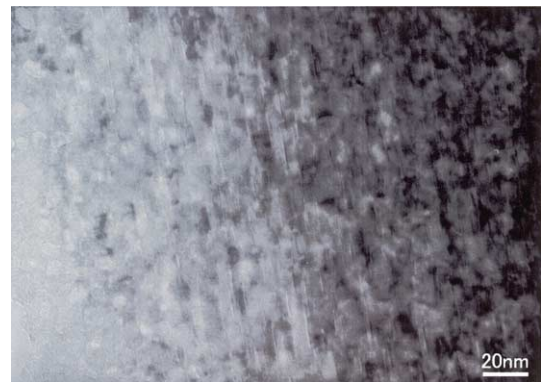
Fig. 4. High-magnification electron micrograph of the as-irradiated Al 14 N specimen showing dislocation loops.
